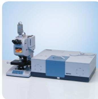
VERTEX 70v and HYPERION 2000 IR microscope. Up to five beam exit ports are available for multiple external modules.
