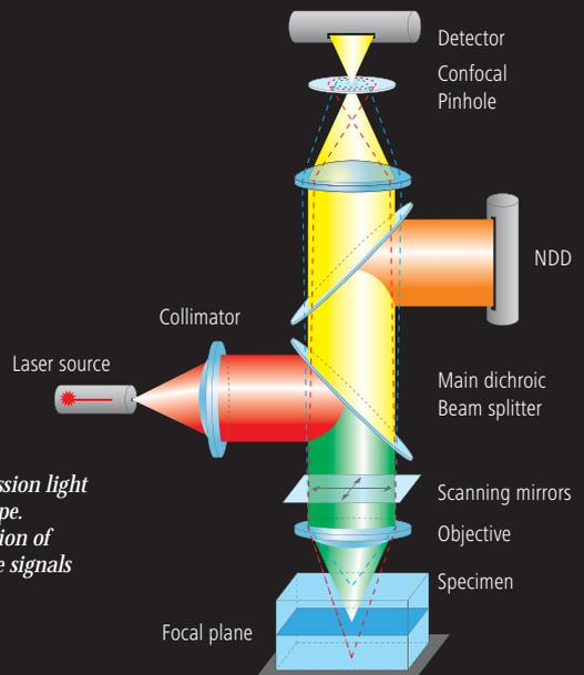
*Beam path of the excitation and emission light in a confocal laser scanning microscope. The confocal pinhole allows the creation of optical sections by hiding fluorescence signals of non-focal levels.*
