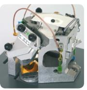
RockSolid™ interferometer used in the VERTEX 70v FTIR spectrometer
