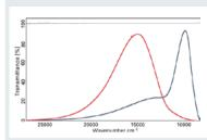
Background and 100%-line (top) measured in the visible spectral range using 8 cm<sup>-1</sup> resolution, 30 sec measurement time, 2 mm diameter aperture and tungsten source, visible beamsplitter and Si-diode detector. By using an optical filter the short wavelength efficiency (red curve) can be significantly improved.
