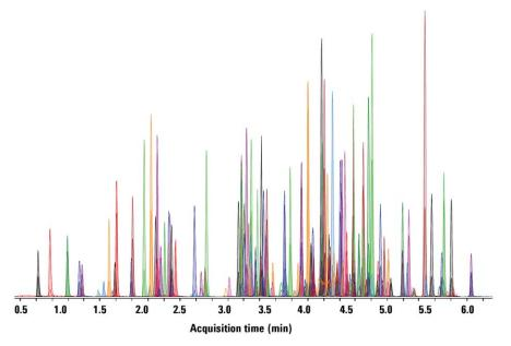
Figure 1. dMRM analysis of 224 pesticides at the 500 parts per trillion level in less than 7 minutes.
