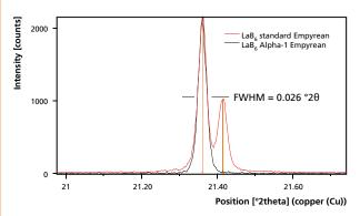
Empyrean sets the new bar for laboratory X-ray system resolution, with a FWHM of 0.026 degrees 2theta for the first reflection of NIST SRM660a LaB $_6$ .
